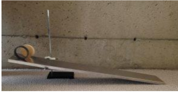
Figure 13: Two objects of the same mass and size (but differently shaped) race down the inclined plane. Which object wins the race?
