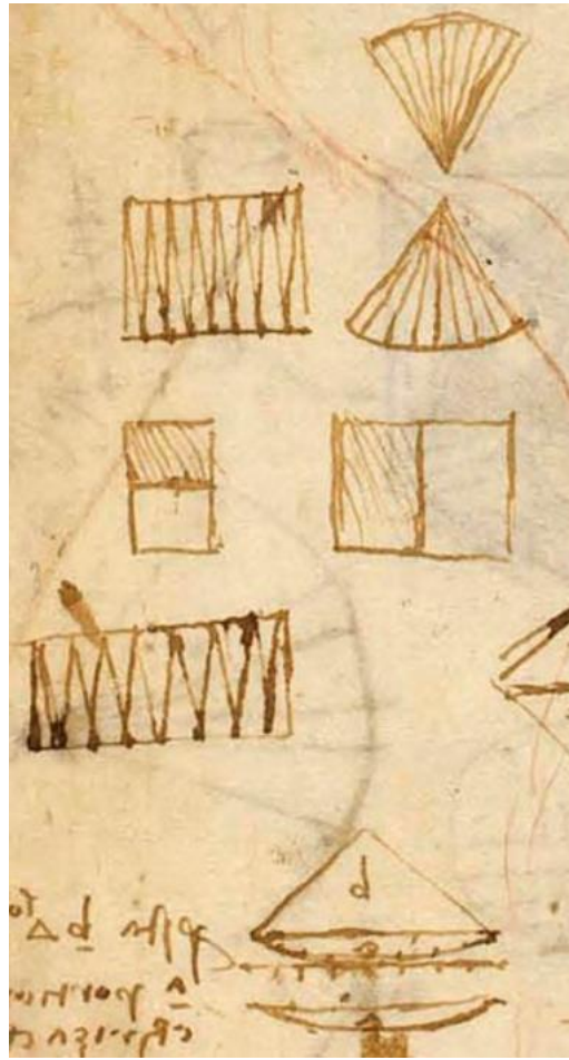
Figure 3: Diagrams from Leonardo da Vinci’s Codex Atlanticus , p. 518 verso. Calculation of the area of a sector. The sector is subdivided into eight smaller ones, then its identical copy is attached to it in order to form a rectangle (da Vinci, 1513).
