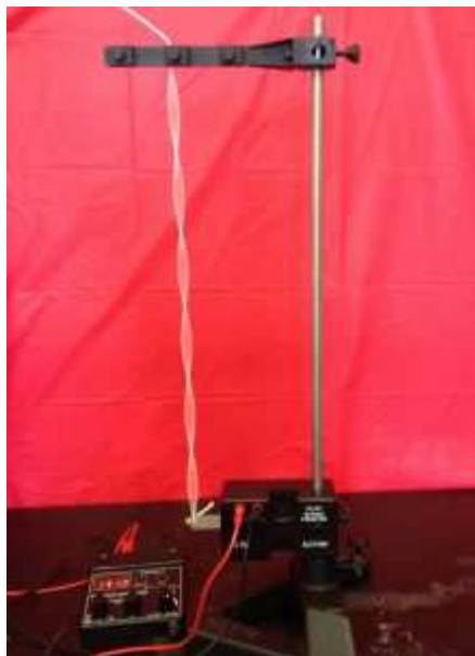
Figure 5. Vibrations in a string. The string is fixed at both ends and the vibrations are caused by a wave generator (rectangular black box near the bottom left).
